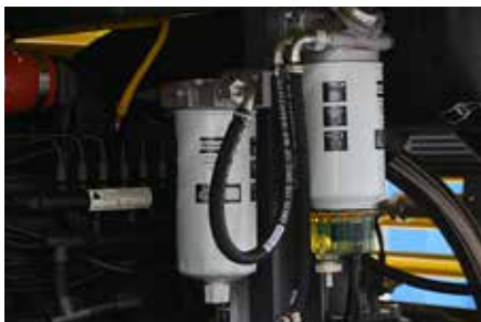
Additional fuel filter as standard to ensure engine protection.
